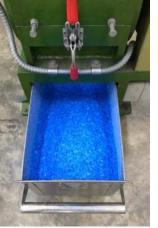
Fabrication of light-weight composites with neutron shielding properties. The composites were successfully prepared from recycled HDPE pellets made from discarded fishing nets and boron carbide. The prototype product from this project will be used for internal utilization at TINT's neutron imaging laboratory.
